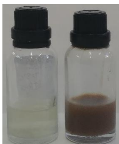
Figure 28: Picture of the raw leachate (right flask) and the leachate after the CWPO (left flask) using HTC-230 under the following experimental conditions: T = 80 \text{ }^\circ\text{C} , pH = 3.00 \pm 0.02 , C_{Catalyst} = 7.2 \text{ g L}^{-1} , V_{Leachate} = 25 \text{ mL} , C_{H_2O_2} = 85.71 \text{ g L}^{-1} in five stepwise additions of 17.14 \text{ g L}^{-1} . *Leachate after the TP-207 pretreatment
