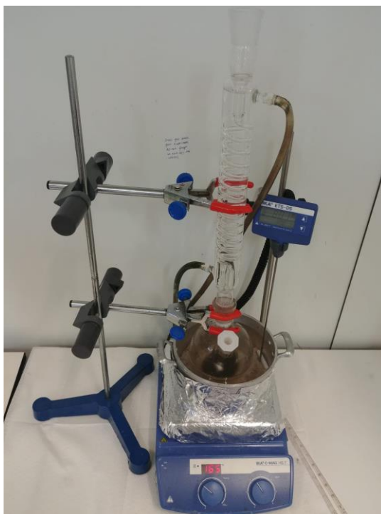
Figure 6: System used for the CWPO runs
